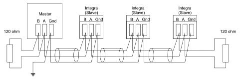
There must be no more than two wires connected to each terminal, this ensures that a "Daisy Chain or "straight line" configuration is used. A "Star" or a network with "Stubs (Tees)" is not recommended as reflections within the cable may result in data corruption.
